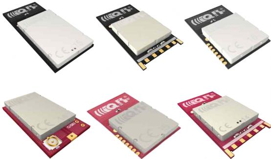
Basic component for RF communication on the IQRF® platform.
